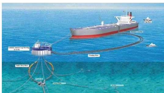
Figure 12: Single Point Mooring (SPM) with Double Pipeline
